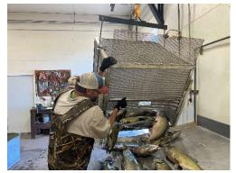
We move about 25 fish at a time (3-400 lbs) with the help of an electric winch. The fish are dispatched in bubbled CO2 prior to spawning.
